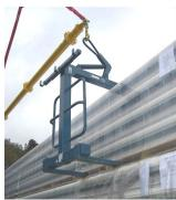
When positioning the Pack Boy<sup>TM</sup> in the panel pack, pay attention to load balance and ensure that the crane forks are fully inserted into the pack up to the heel of the forks. The use of push rods to aid insertion of the forks into each pack will avoid the need to climb on the delivery vehicle.
